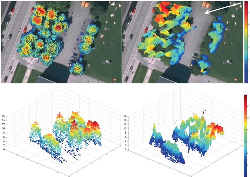
Fig. 7: Top row: Two-dimensional representation of LiDAR point cloud (left) and InSAR point cloud (right). Note how many parts of the InSAR tree heights are affected by layover. The white arrow shows the SAR viewing direction. Bottom row: Three-dimensional view of LiDAR point cloud (left) and InSAR point cloud (right), approximately from the SAR perspective.
